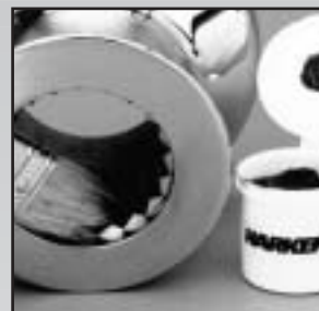
Grease gear teeth lightly.
