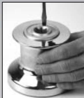
Use screwdriver to open winch.
