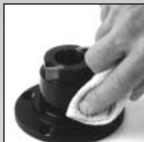
Clean all parts with solvent.
