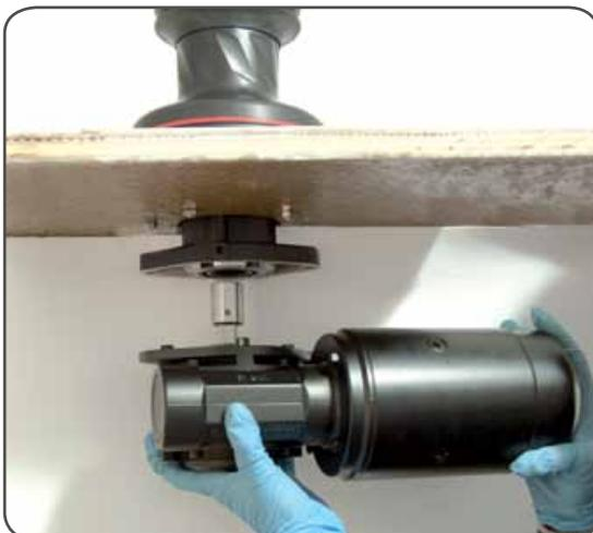
3. Position the reduction gear and motor
