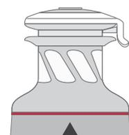
After correctly positioning the final drive gear with respect to the load, check that the motor, gearing, electrical wiring and/or hydraulic pipes can be housed below decks. To help find the optimal compromise, remember that, to make the installation of the motor easier, it can be coupled to the winch in any one of four different positions that differ by  $60^\circ$  from each other.
