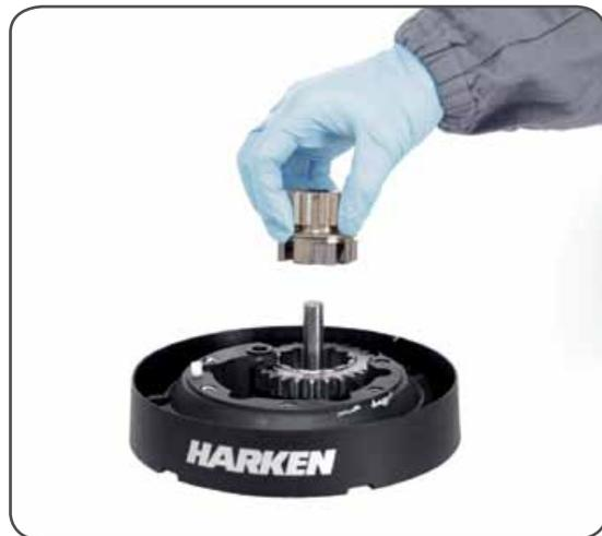
16. Remove the pinion n°11. To facilitate the operation press the spring against the pawl with a blade
