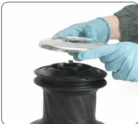
5. Remove the stripper arm n°28 by rotating and lifting it.
