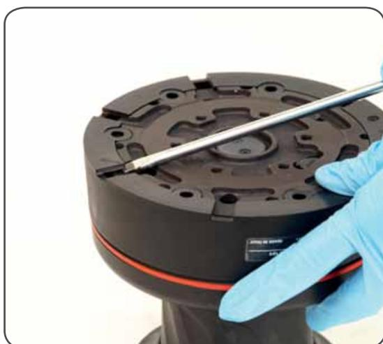
1. Remove the skirt n°2 with the help of the screwdriver placed as shown by the symbol
