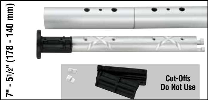
7" - 51/2" (178 – 140 mm) Do not use plastic bushing above top connector. Shorten top of connector and if necessary shorten trim cap.
