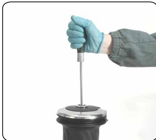
2. Unscrew the central screw ( \approx 2\text{Nm}/18\text{ in-lb} )
