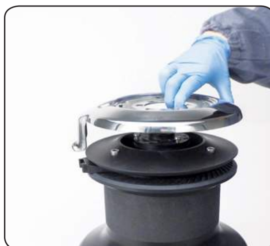
5. Unscrew the three screws n°37 ( \approx 4\text{Nm}/35\text{ in-lb} ) and remove the stripper arm n°36 by rotating and lifting it.
