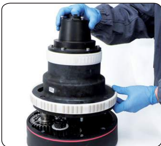
8. Lift off the assy housing n°18
