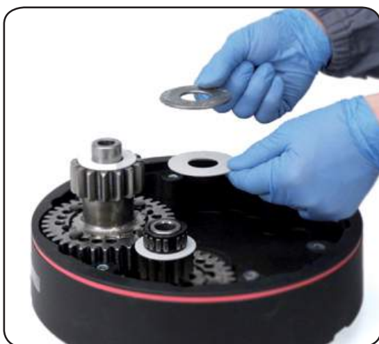
14. Remove washers n°30 and n°29. Important: The plastic washer must be positioned in contact with the winch base.
