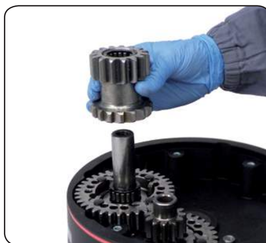
17. Slide out the final drive pinion n°9
