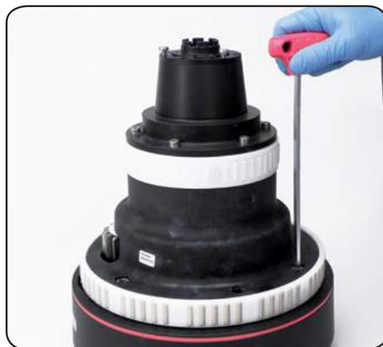
7. Completely unscrew the six screws n°25 ( \approx 20\text{Nm}/177\text{ in-lb} )
