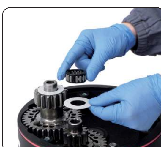
15. Slide out the roller bearing n°6 and the washer n°5
