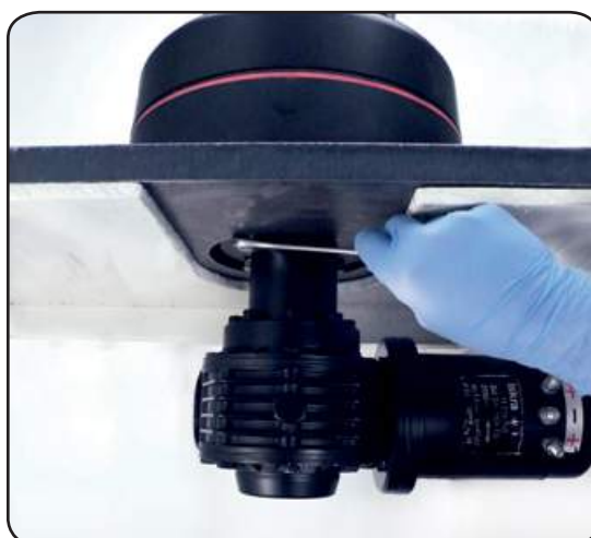
2. Tighten four M6 precote coated screws (8 Nm/ 71 in-lb)
