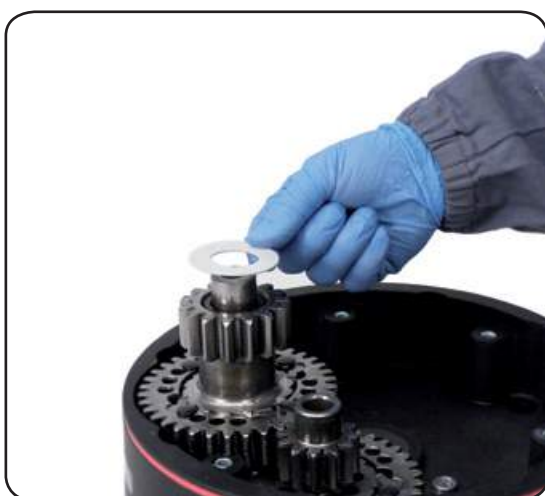
16. Slide out the washer n°5
