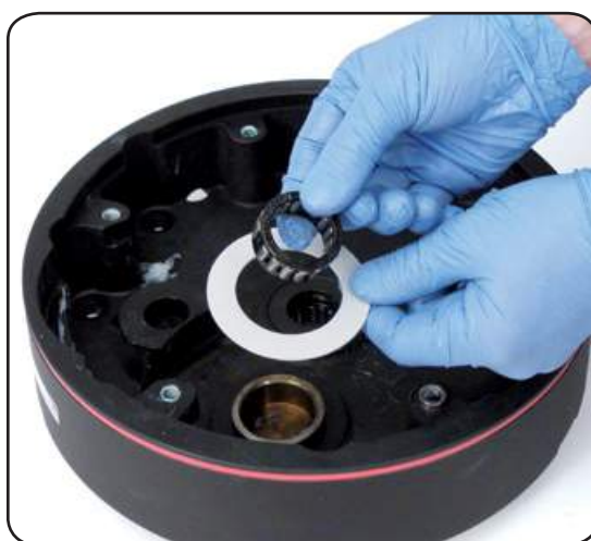
23. Remove the roller bearing n°6 and the washer n°11
