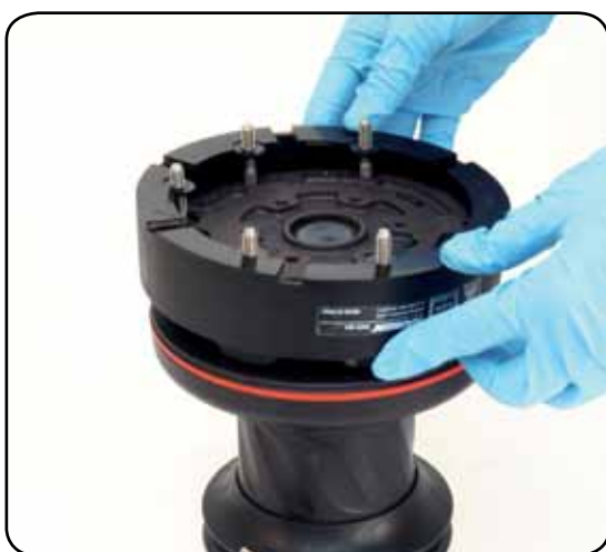
4. Reposition the skirt n°2 in its housing
