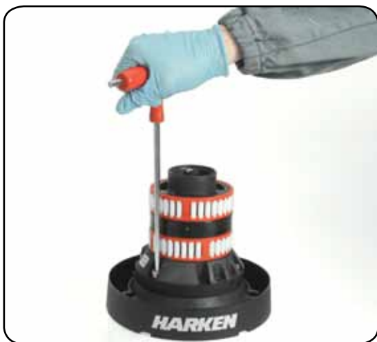
8. Unscrew the 5 hex screws n°18 (20Nm/177 in-lb)
