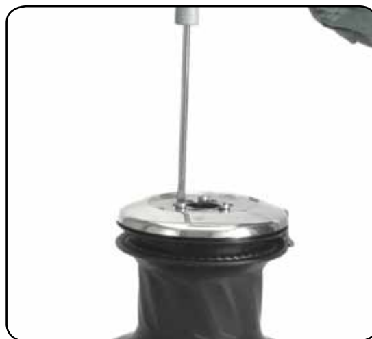
4. Unscrew the three screws n°29 ( \approx 4\text{Nm}/35\text{ in-lb} )
