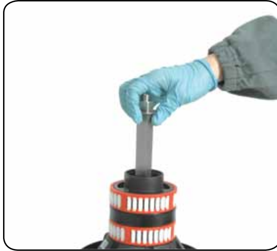
7. Slide out the central shaft n°21
