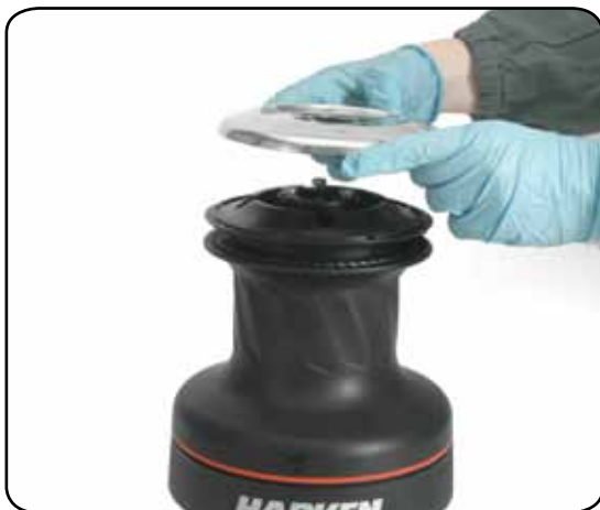
5. Remove the self-tailing arm n°28 by rotating and lifting it.
