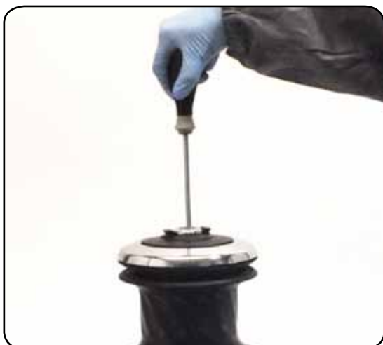
1. Unscrew the central screw (🔧 2Nm/18 in-lb)
