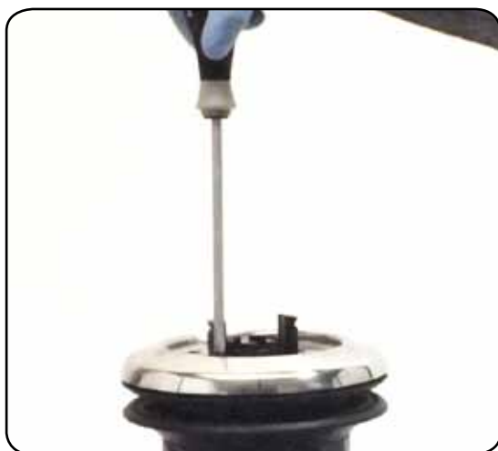
3. Unscrew the three screws n°28 (🔧 4Nm/35 in-lb)
