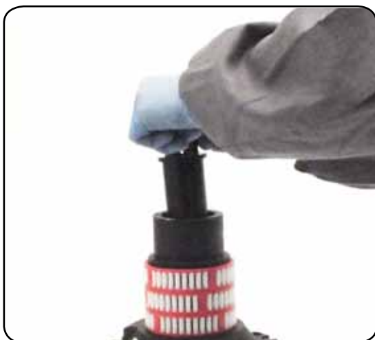
7. Slide out the assy clutch n°37
