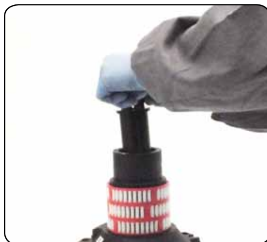
7. Slide out the assy clutch n°37
