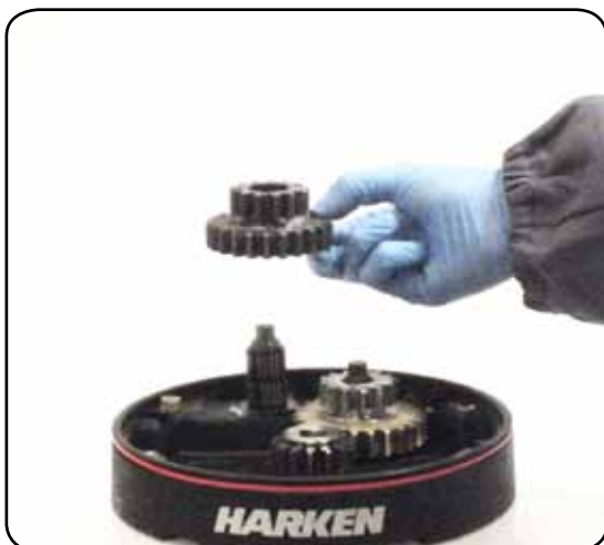
13. Remove the idler and pinion n°14
