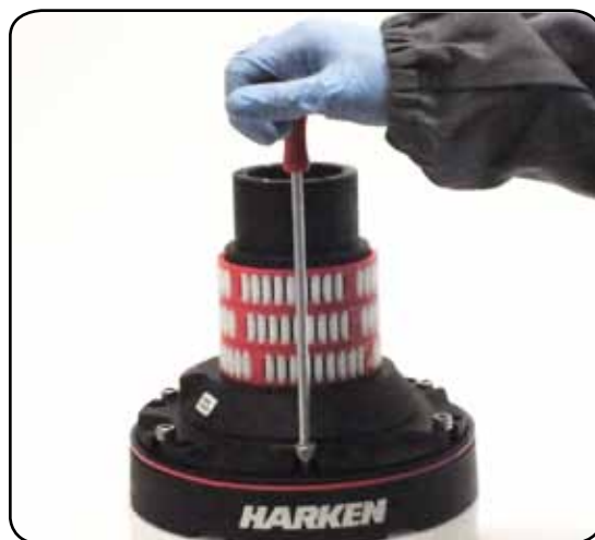
9. Unscrew the 6 hex screws n°17 ( \hookrightarrow 20Nm/177 in-lb)
