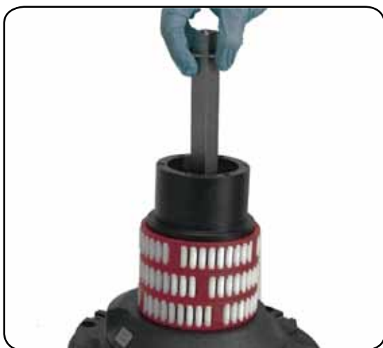
8. Slide out the central shaft n°19
